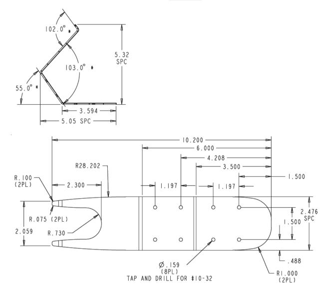
Measurements: MOUNTING BRKET SMALL 7400VB, RAM-B-101U (adjustable mount) PN# 8000046
